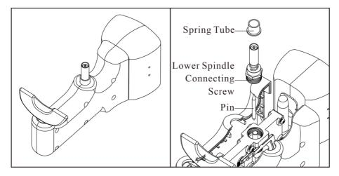
When the tester is used over a longer period of time, especially when measuring soft aluminium alloy materials, some material might remain on the pin which might affect the accuracy of the device. To eliminate this error, make sure to check and clean the top of the measuring pin on a regular basis.
