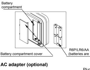
AC adaptor socket R6P/LR6/AA size dry batteries. (batteries are not included)
