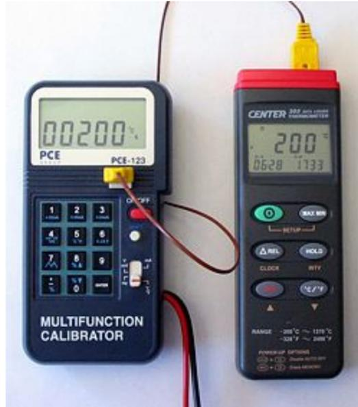
**Digital, electrical, current, voltage or process calibrator, tester or multimeter for simulation and measurement of standardized electrical signals / control signals as well as frequencies and temperature**
