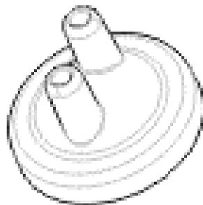
1. To fit the flow cap, slip the flow cap over the sensor on the front of your Gasman unit, until the cap is tightly fitted into place.
