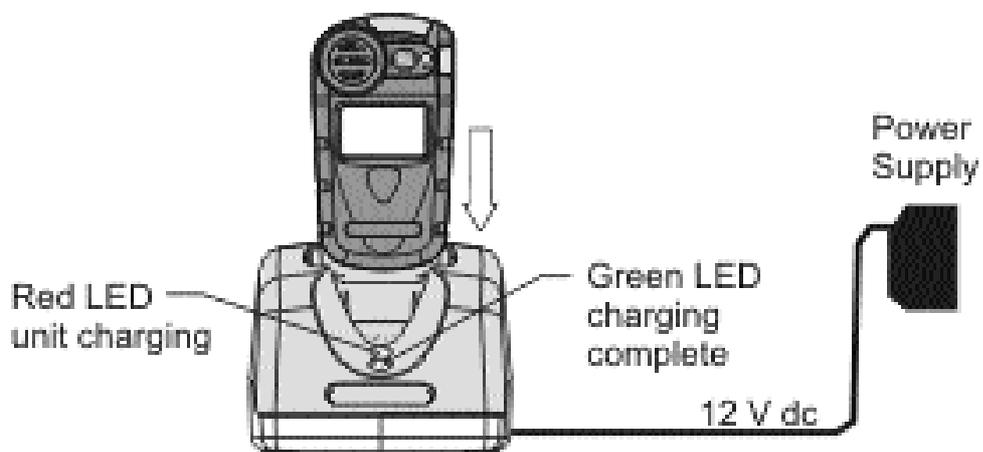
The Gasman unit would normally be left switched off for charging and will display a battery icon on the display screen sweeping from empty to full. During charging the red LED on the front of the charger unit will be lit. When charging is complete, the green LED on the charger unit will illuminate.
