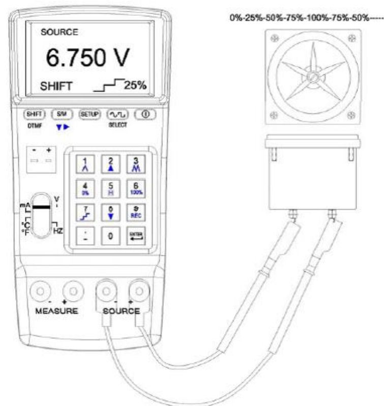
Connection for multistage sampling
