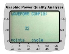
**NOTE:** The unit will adjust the sampling time according to the processing time required to log waveform.
