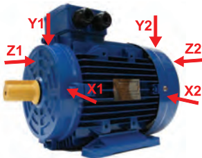
Figure 15: Measuring points on electric motors
