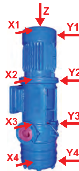
Figure 16: Measuring points on machines with vertical rotors
