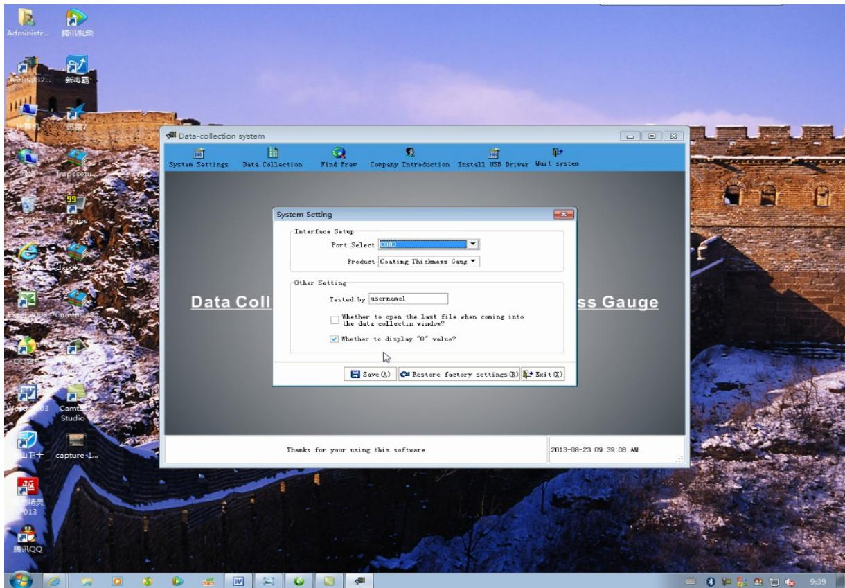
After using the instrument to obtain measurements, connect the instrument to the computer using the custom cable provided. Open the software and click data collection to enter the acquisition interface. Then click new to start downloading the measurement data.
