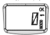
The sensor channel will display the current value of the gas being monitored and units of measurement, the 'OK' symbol will flash indicating unit is working correctly. Familiarise yourself with the gas currently being monitored in your unit. Ensure you understand site health and safety procedures. For information on Peak and TWA readings, go to section 2.4.
