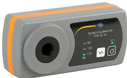
Turn on the sound level meter and set it to A weighting, fast response and a range of 70 ... 130 dB. Carefully insert the microphone into the 1/2 inch hole of the calibrator set to 94dB @ 1kHz. Adjust the calibration potentiometer with a small screw driver. Reattach the back cover.
