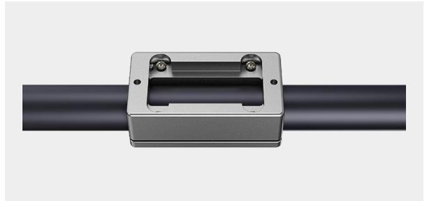
Align flow meter to the pipe position, install screw on top part of the bracket, and then the bottom part of the bracket will automatically connect with the top part. Fasten the four M4 screws.
