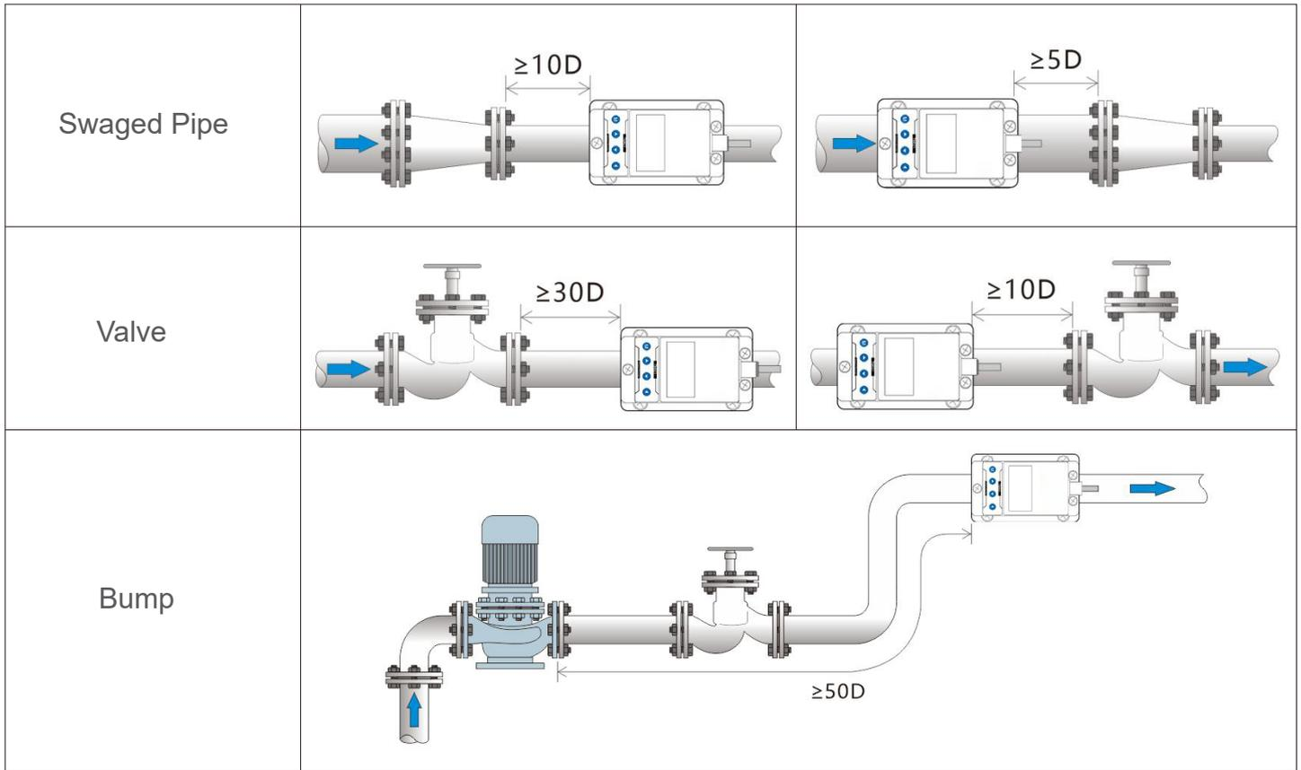
Note: D refers to the diameter of the pipe, such as: the pipe is DN25, 10D is 254mm
