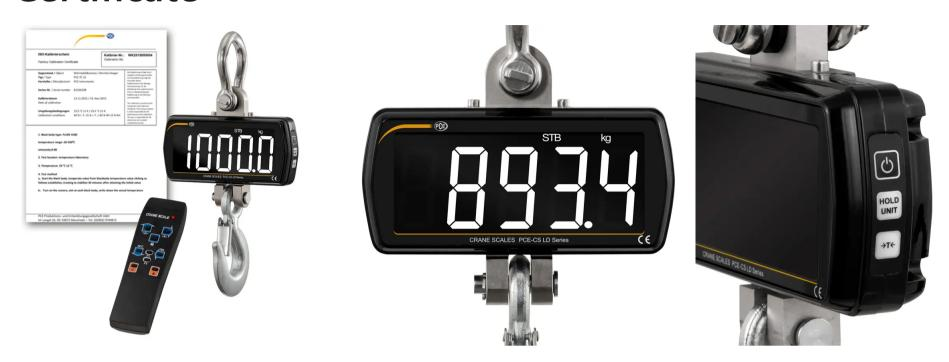
Hanging scales with remote control / Measuring ranges 0 ... 1000 kg (0 ... 2205 lbs) / Metal housing /Various units of mass / With hook and shackle / Large LCD display / Battery operation / Shackle opening 23 mm / Summing function / Incl. ISO calibration certificate
