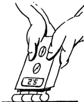
The instrument is equipped with an automatic power off which activates 5 minutes after the last change in upper control knob setting. Moisture meter can also be switched off instantly by setting the upper control knob to OFF.
