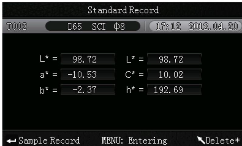
Here you can navigate between the different readings by using the arrow keys ( $\blacktriangleup$  and  $\blacktriangledown$ ).
