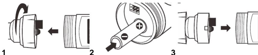
1. Unscrew the union nut of the electrode and pull the electrode off the measuring device, observing correct axial alignment.
