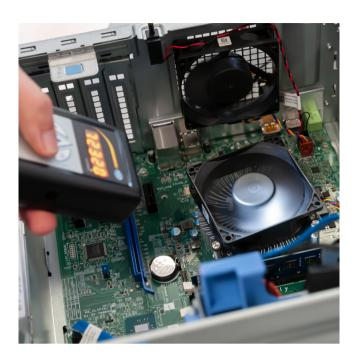
LED Tachometer / Light and compact / 60 ... 99,990 flash/ Min range / One handed operation with 6 keys / 2 very bright LEDs (1400 lux @ 50 cm) / Duplication and division of impulses / Tripod connection
