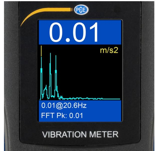
**Vibration analyzer with 4 GB data memory / FFT analysis / Waveform display / Infrared temperature meter / Measuring range 0 ... 200 mm/s<sup>2</sup> / Battery life of 8 hours /
