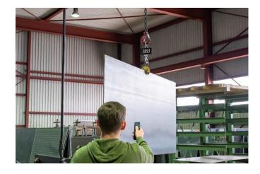
The compact hanging scales work well in areas where large and bulky parts need to be weighed. They are light and compact so that they can be carried quickly and easily to another attachment point. Nevertheless, the metal housing is very robust and resistant. The energy-saving technology enables an operating time of approx. 45 hours with one set of batteries.
