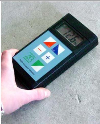
A hand holds the FMW-B moisture detector against a grey concrete surface. The LCD screen displays '12.6%'. |
