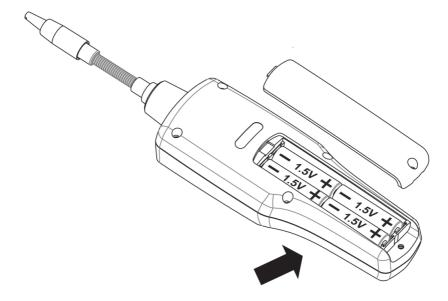
To supply power from batteries, open the battery compartment on the back. Then insert four 1.5 V AA batteries. Ensure correct polarity when inserting them. After inserting the batteries, close the battery compartment.
