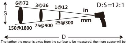
I he farther the meter is away from the surface to be measured, the more space will be measured. If the distance-to-spot ratio is too large, undesired surfaces may be included in the measurement. This will cause incorrect readings.
