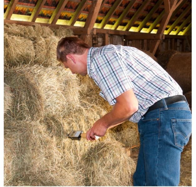
**Hay hygrometer to determine moisture and temperature of hay and straw / Robust design / Four different lengths of measuring lance of 25 cm, 50 cm, 100 cm or 270 cm / Continuous display of measuring value**
