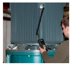
The compact and robust vibration data logger PCE-VT 3900 with route measurement, FFT analysis and extensive memory options is particularly suitable for the repeated monitoring of vibration-prone machines and components in extensive systems. Thanks to the versatile evaluation options of the PCE-VT 3900, conspicuous vibration values can be quickly detected, reliably documented and correctly evaluated.
