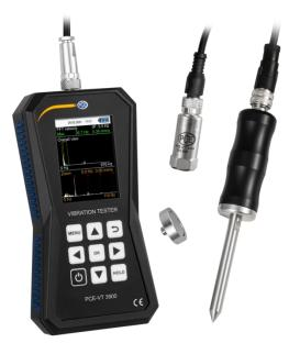
displacement. The current measured value can be displayed as an effective value (RMS), peak or crest value, peak-to-peak value (value between the highest and lowest reading) or as a crest or peak factor (quotient of peak and RMS).
