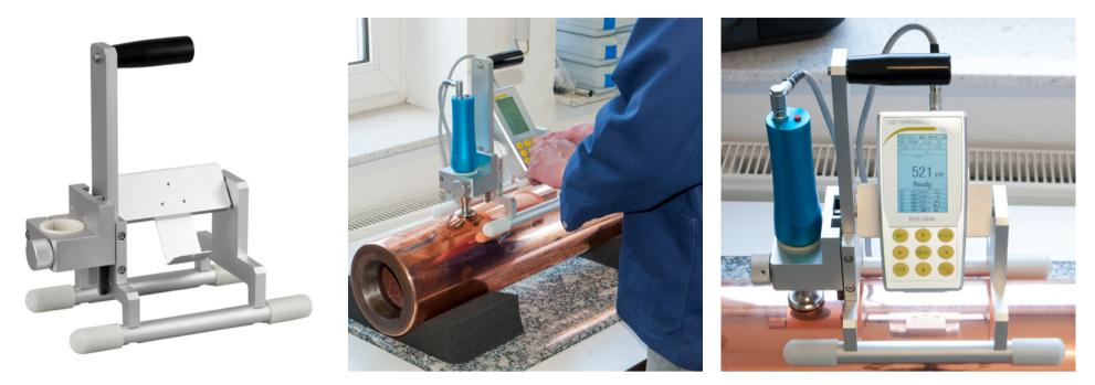
The PCE-5000-STAND test stand for the PCE-5000 hardness tester is used to support the automatic test probes. The test stand allows automated measurements, with a higher reproducibility of tubes and round material. The test stand can, of course, be used for flat surfaces.
