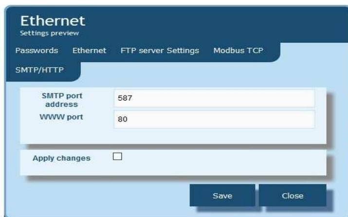
*Fig. 20 View of SMTP port configuration window on "Ethernet" tile*
