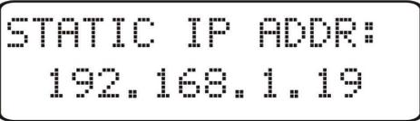
b) message about the monitor operation with a DHCP client disabled – the displayed IP address is the current address of the monitor set manually or the default address (after restoration of default parameters); in order to obtain an address
