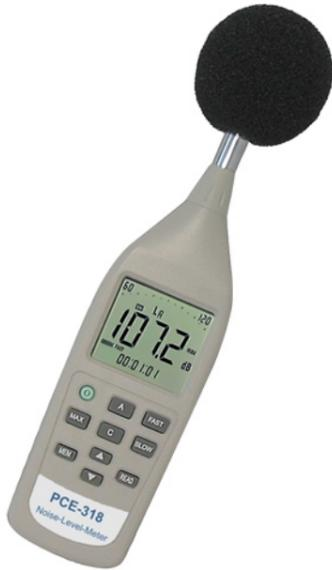
**Sound level meter PCE-318 with a range between 26 ... 130 dB (A) and an analog output/ recalibrated / Class II (accuracy  $\pm 1.5$  dB)**
