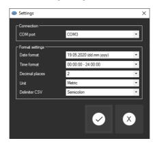
In addition to the connection data, some format settings for the software can be made here, including the date format, the time format and the way the statistical values are displayed. You can also select a delimiter which is used when a series of measurements is exported into a CSV file.
