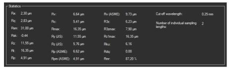
The statistics show the most important R parameters as well as two settings regarding the measurement (number of individual sampling lengths and cut-off wavelength).
