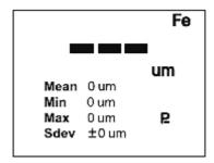
The  ${\bf P}$  icon means that the thickness measured is beyond the measuring range or the meter has failed to measure.
