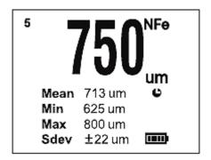
The cicon means the device will be powered down in 3 seconds.
