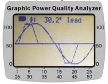
Users can press the +▶or -◀ buttons to move the 0 reference axis of current up or down. So the waveforms of voltage and current can be easily distinguished as in the following figure.
