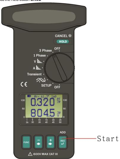
Users can press the REC button once to start scheduled datalogging. The **START TIME** and **STOP TIME** is set in the SETUP.
