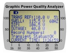
It shows the reference voltage is AC 110.0V (**TRANS REF**), and the threshold is 5%. If the voltage exceeds 115.5V (**SWELL**) or is less than 104.5V (**DIP**), or is less the 40.0V (**OUTAGE**), one transient event will be logged.
