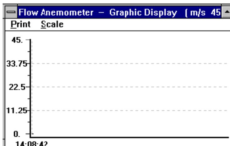
If this option is selected or CTRL+G is pressed, a window, which emulates strip chart recorder, shall appear on the screen. The graphic window has two menus, PRINT and SCALE. Select the PRINT menu, the graphics will be printed through any printer connected to the PC. The SCALE menu allows user to set the minimum and maximum value for the Y (vertical) axis.
