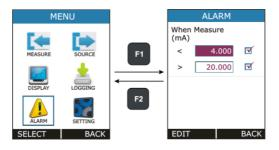
Individual alarm limit values may also be enabled/disabled using the check box preceding the alarm limit value. To stop the alarm, uncheck the appropriate alarm checkbox.
