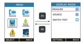
There is mainly Four RUN Display Mode possible in this device. And this mode can be selected from the above Page. What information to be shown in each RUN Display Mode can be defined by this page.
