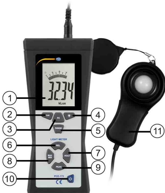
1. LCD Display: 3-3/4 digit displays with a maximum reading of 3999, and the indicating signs of measured values, unit function symbols and decimal points etc are display.
