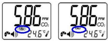
The gas detector should be calibrated at least every two years. To do so, you can use the ambient air outdoors. The housing needs about 10 minutes to acclimate. Wait until the  $CO_2$  reading on the display is stable. The display should indicate between 380 and 420 ppm.
