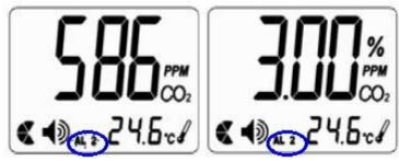
To adjust the AL2 threshold level, press the "Mode" key until "AL2" appears on the display and press "Enter" to confirm. Now you can switch between the available options by pressing the "Mode" key. The following options are available: 1.5 %, 2 %, 2.5 %, 3 %, 3.5 %, 4 %. Select the desired option and press the "Enter" key to confirm.
