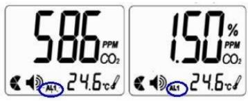
To adjust the AL1 threshold level, press the "Mode" key until "AL1" appears on the display and press "Enter" to confirm. Now you can switch between the available options by pressing the "Mode" key. The following options are available: 0.5 %, 1 %, 1.5 %, 2 %. Select the desired option and press the "Enter" key to confirm.
