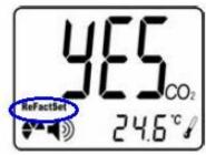
Using this function deletes all stored settings and sets the device back to factory default settings. This might be reasonable if the calibration has not been done properly, for example.
