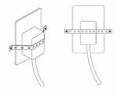
Connect the mains adaptor to the wall socket. Attach the elastic safety strip to the power plug by using screws and wall plugs. The strip should sit so tight that the plug cannot be pulled out of the socket without using mechanical tools. Once the mains adaptor is connected to the power source, the Sensor unit and the remote display unit start monitoring.
