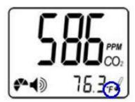
To switch between "°C" and "°F", press the "Enter" key.
