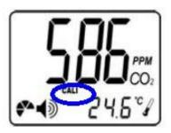
The gas detector should be calibrated at least every two years. To do so, you can use the ambient air outdoors. The housing needs about 10 minutes to acclimate. Wait until the CO<sub>2</sub> reading on the display is stable. The display should indicate between 380 and 420 ppm.
