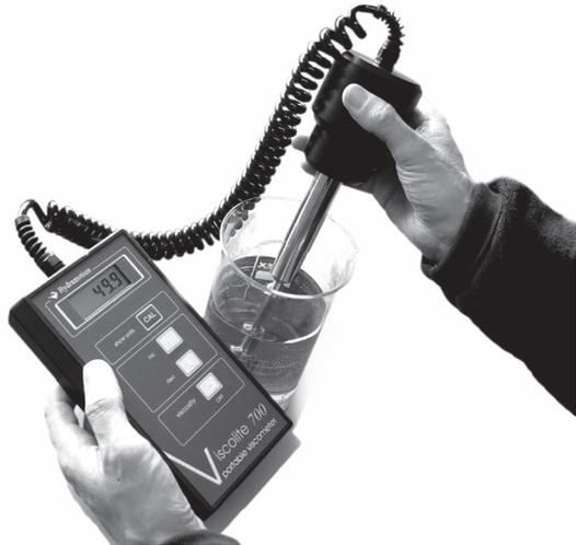
**The Viscolite® VL7 is an easy-to-use portable instrument for the instant measurement of viscosity anywhere at any time using a simple dip-in probe. No prior setting-up or adjustment is required.**
