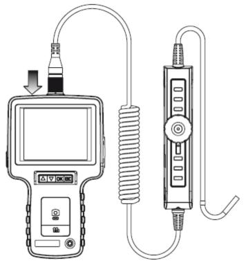
Connect the connecting cable to the display unit of the endoscope and screw it tightly. Make sure that the indication on the connector is on the upper side.
