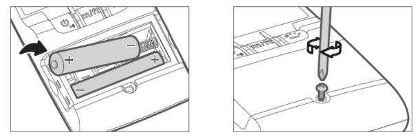
The battery compartment of the cable measuring device is located at the front, right below the function keys. To open it, you have to loosen a screw first. After that, you can open the battery compartment and replace the batteries.
