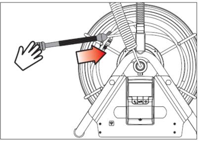
1. Hold the camera head horizontally and carefully coil up the cable.
