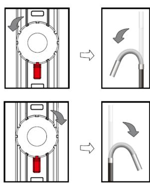
2. You can lock the pivoting angle of the camera head by using the red locking lever. To lock the camera head, carefully push the lever clockwise all the way to the stop. To unlock the camera head carefully push the lever counter-clockwise, until it reaches its starting point.
