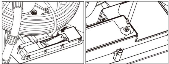
The battery compartment of the transmitting unit is located at the back of the unit. To open it, you have to loosen a screw first. After that, you can open the battery compartment and replace the batteries.
