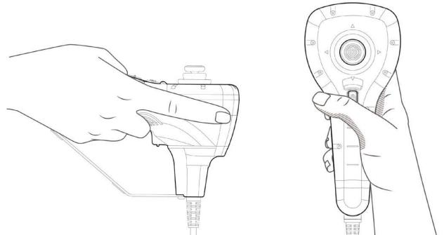
Hold the device with one hand and use your thumb for operating the joystick and the function keys. With your index finger, you can use the boost key.
