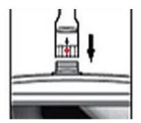
Connect the camera cable to the display unit and screw it tightly. Make sure that the indication on the connector is on the upper side (see picture above).
