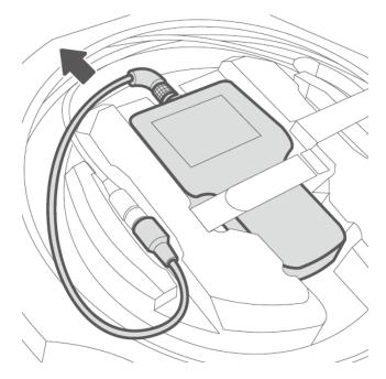
Insert the display unit into the carrying system as seen in the picture above. Use the connecting cable to connect the display unit to the camera tube, Roll up the camera tube on the carrying system.
