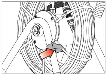
1. Before pulling out the camera cable, loosen the cable drum fixing first.
