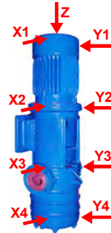
Figure 12: Measuring Points on Machines with Vertical Rotors
