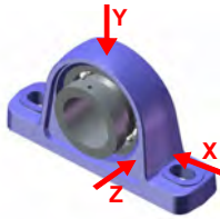
Figure 9: Measuring Points on Vertical Bearings
