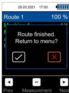
Fig. 37 Route measurement completed
