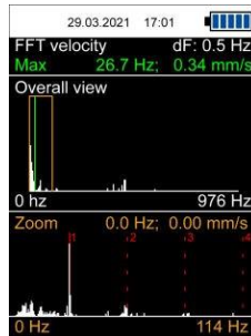
Fig. 42 Display of harmonics
