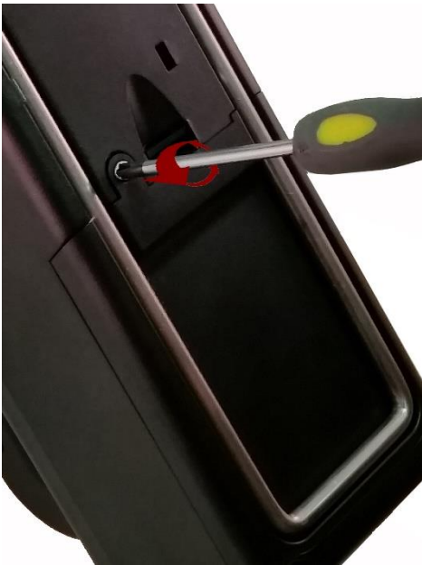
Step 1 - Remove security screw with Phillips screwdriver
