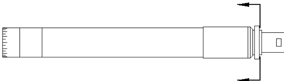
Fig. 5.1. Disconnecting of microphone preamplifier equipped with LEMO connector.
