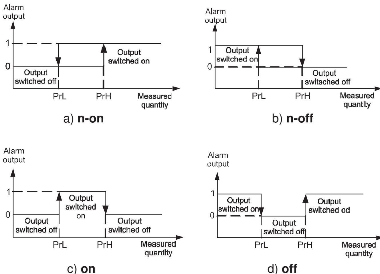
Fig. 11. Tipi di allarme: a) n-on, b) n-off c) on d) off.
