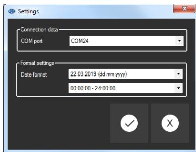
In addition to the connection data, further settings for the date and time format can be made here.
