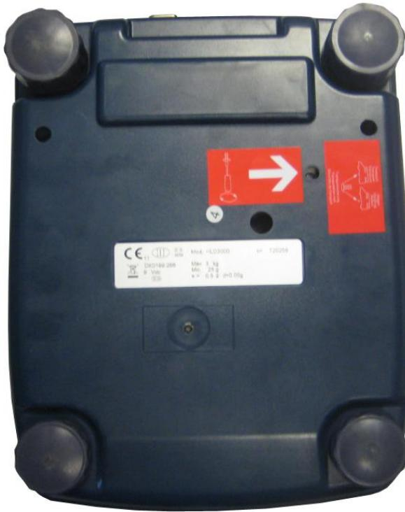
c) Level the platform by adjusting the adjustable feet until the bubble is in the centre of the level. The stability of the platform is very important.
