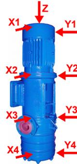
Figure 12: Measuring Points on Machines with Vertical Rotors
