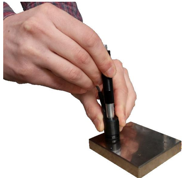
Figure 1.4 – Charging the spring of the probe
