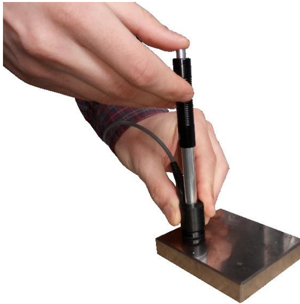
Figure 1.5 – Pushing the trigger button of the probe
