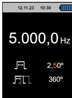
Figure 32. Quick mode - duty cycle modification
