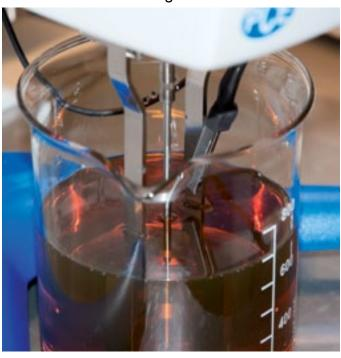
processes the viscosity during mashing can be measured quickly and precisely only with the help of the viscometer.
