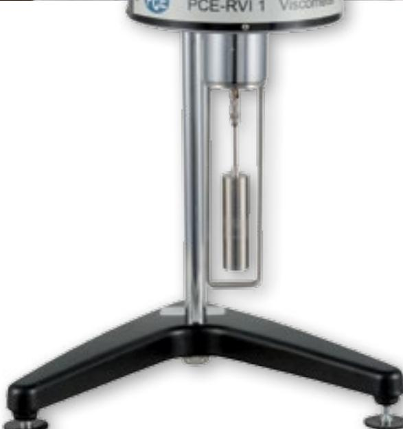
Viscometers are used to determine the viscosity of a fluid. The higher the viscosity value of a fluid, the thicker it is. The elastic capacity of a fluid is called viscosity. There are different viscometers in various designs and with several operating principles. Rotational viscometers as well as Stabinger viscometers use the rotational movement of a cylinder in a sample to determine the torque.
